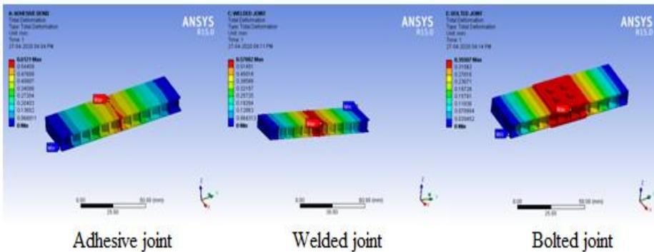
Fig.3: Analysis of deformation in different butt joints
