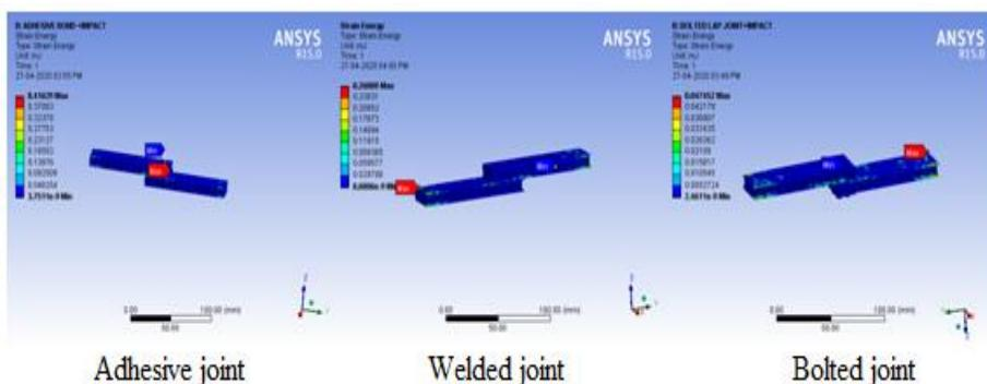
Fig.13: Impact analysis of different lap joints
