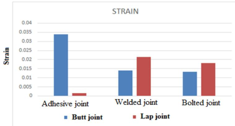
Fig.11: Comparison of strain in various joints of aluminum honeycomb composite panels
