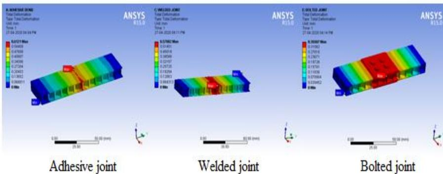
Fig.4: Analysis of deformation in different lap joints
