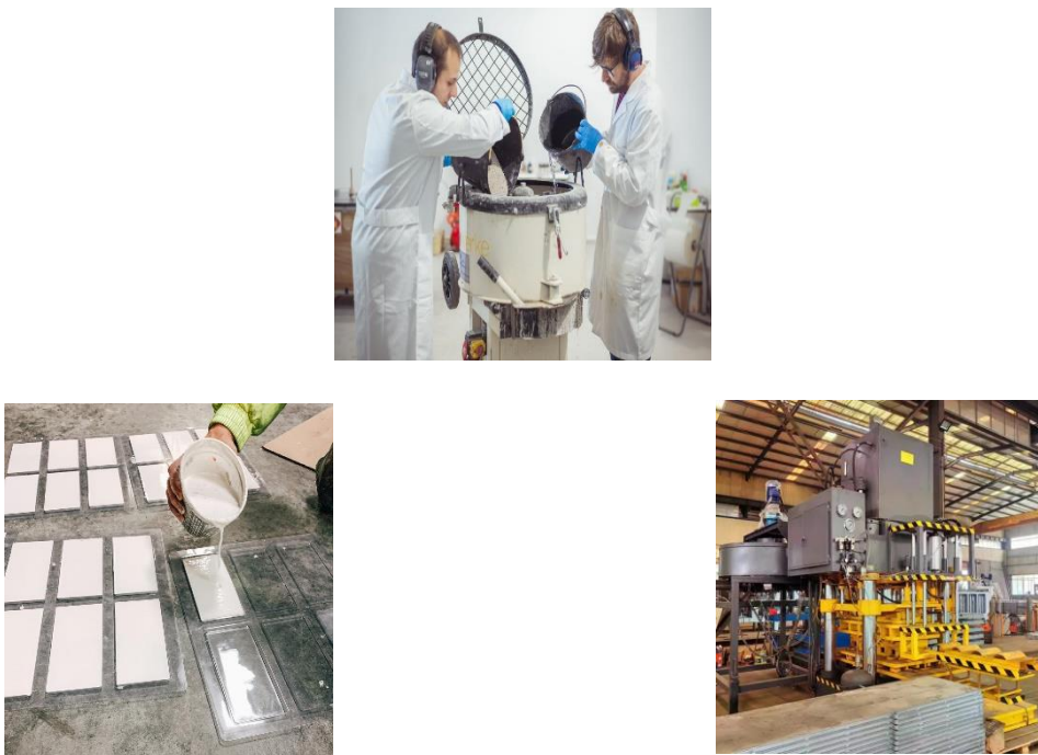
Figure 3. Experimental manufacturing process showing (a) mixing of raw materials, (b) casting into moulds, (c) compaction/pressing, and (d) curing of eco-tiles before testing.
